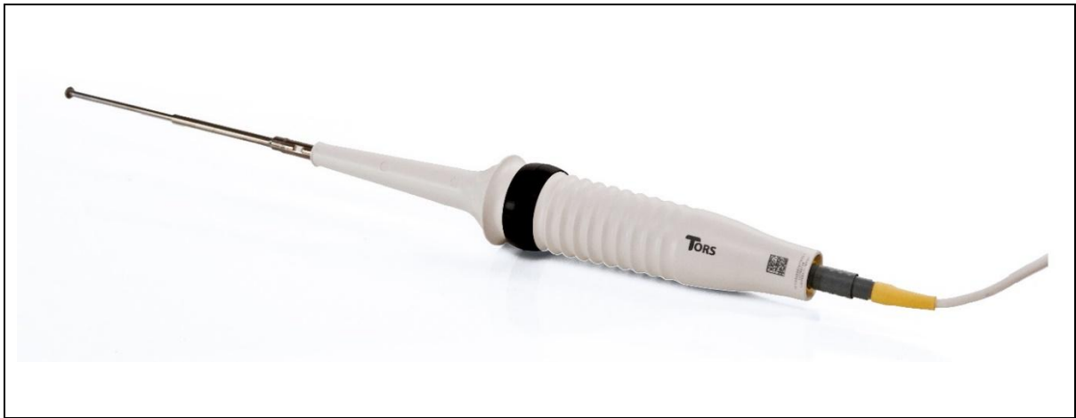
Figure 7 – Axial Grip with TDCR and Probe fitted
